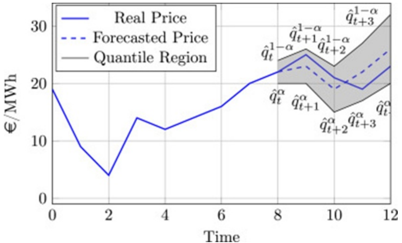
Figure 2. Quantile forecast of electricity prices.
