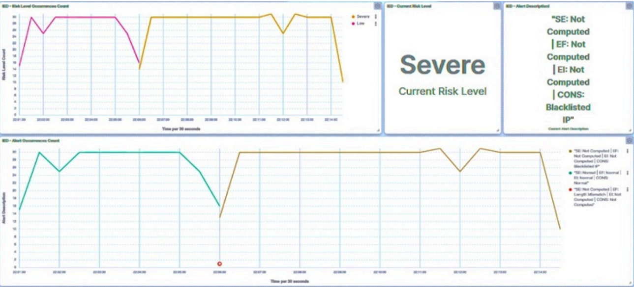
Figure 37. SCADA interface—IED1B stacking detected
