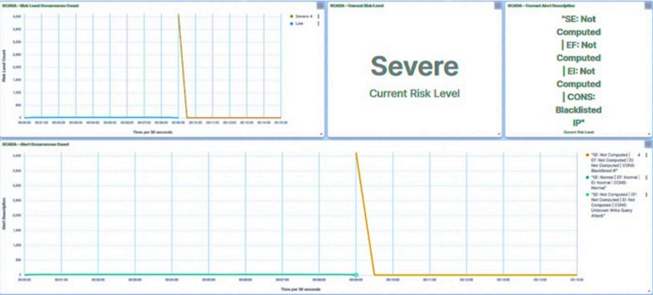
Figure 35. IED4C interface—SCADA brute force I/O detected
