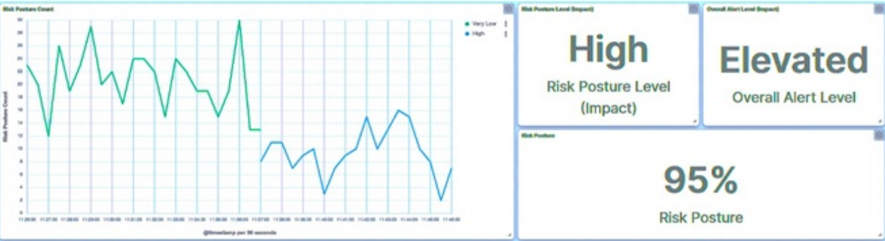
Figure 30. Central agent interface—SCADA replay on IED1A
