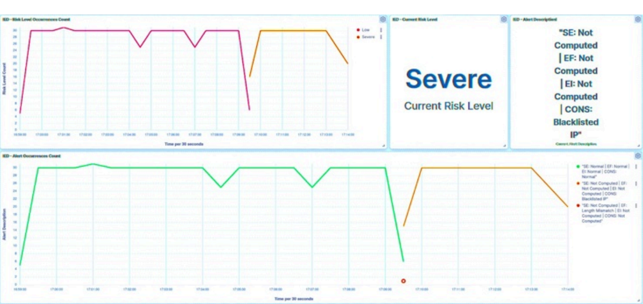
Figure 39. SCADA interface—IED1B length manipulation detected
