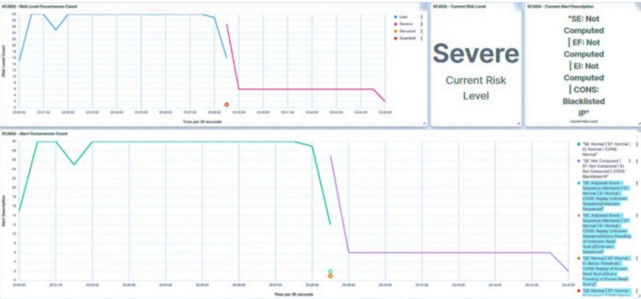
Figure 19. IED1A interface—SCADA flooding detected
