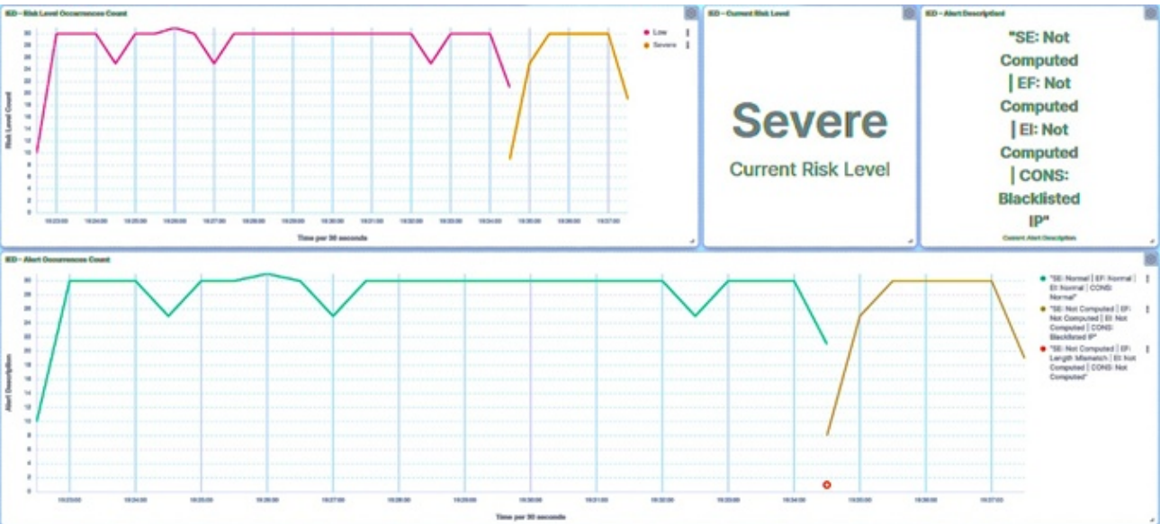
Figure 41. Trust SCADA HMI interface—IED1B payload injection detected
