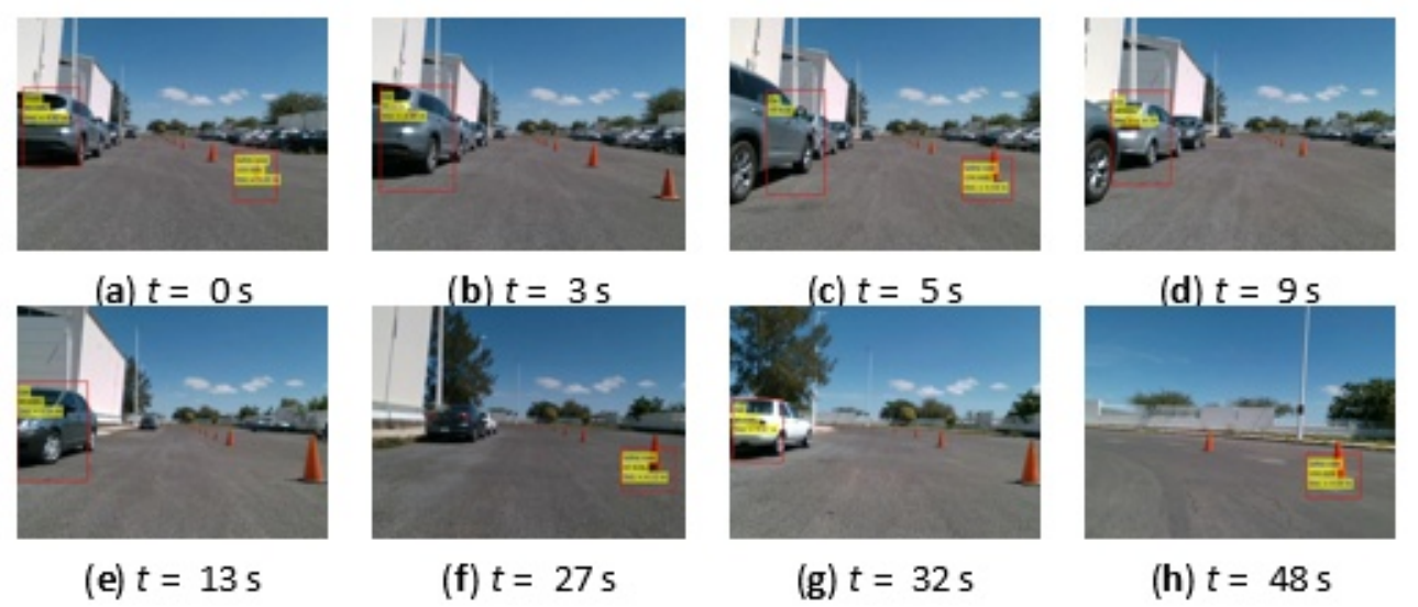
Figure 14. Detection, distance, and classification of objects in a sequence.
