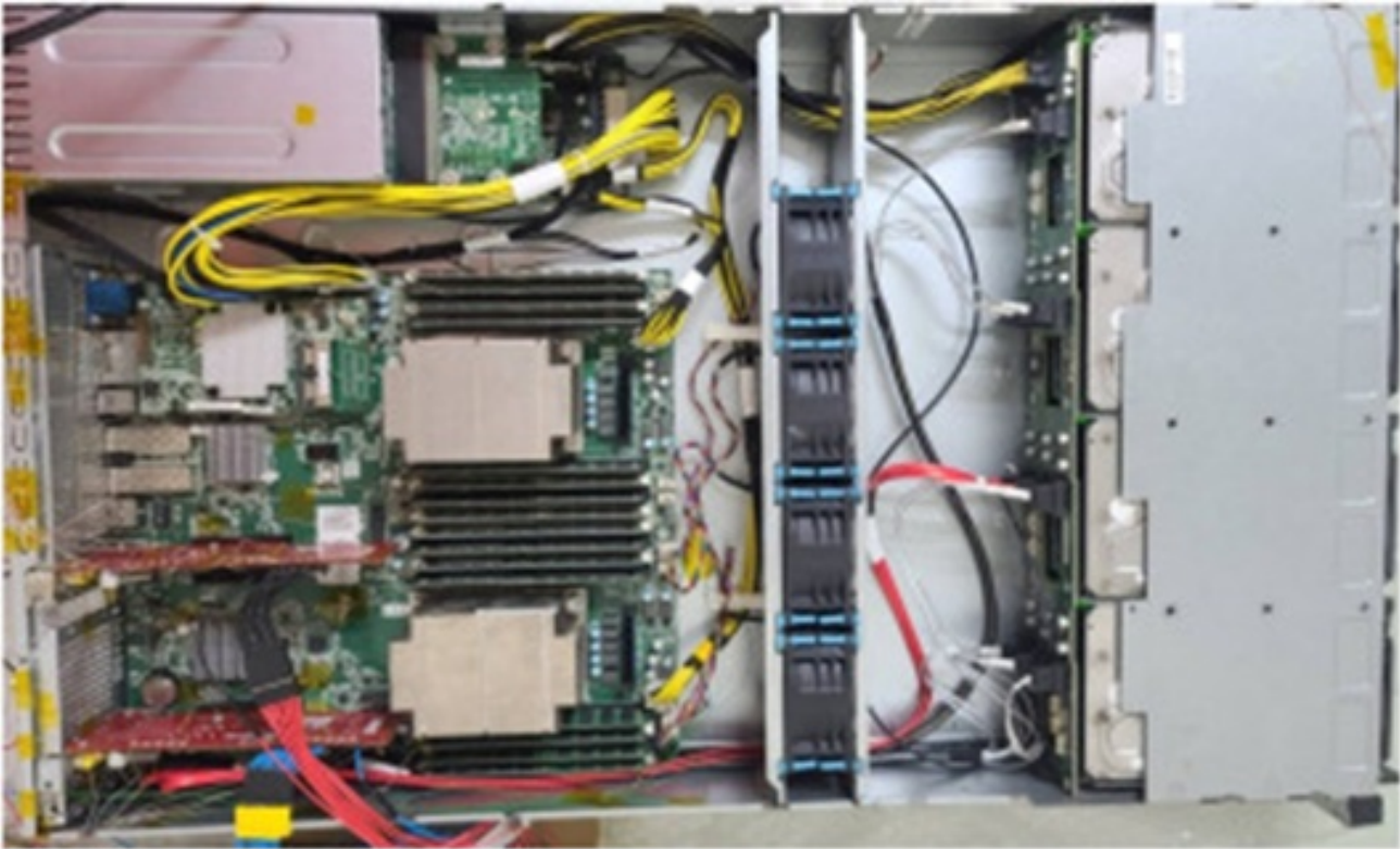
Figure 2. The real location map of the internal components of the server.
